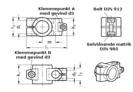
Adjustable clamp lever for d3 = GN 911-M 8-32 have to be ordred separatelyI1 = 81.5Adjustable clamp lever for d4 = GN 911-M 6-25 have to be ordred separatelyI2 = 40
